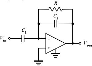
b. Characterize the circuit as LP or HP, and justify your decision by determining values for the low-frequency gain, the high-frequency gain, and the cutoff frequency.
